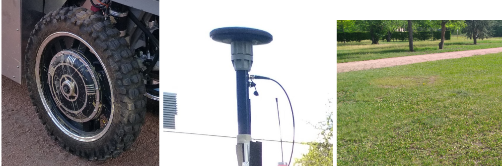
Figure 4.11: Example of sources of influence on the optimal control parameters. Left: wheel, actuator dynamics. Middle: GPS sensor, perception quality. Right: ground, environment.
